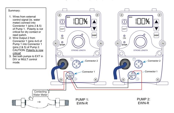
With an EWN-R as the 2<sup>nd</sup> pump, the input terminals (Pins 2 & 5) of Connector 1 are the same as the first pump. The programming of the 2<sup>nd</sup> pump will also have to be set for EXT control mode and programmed for either MULT (for a 1:1 ratio or higher) or DIV (if it is to be run at a fraction of the first pump's speed).
